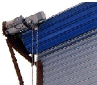
The KJ500, KJ600 and KJ1000 rolling door operators are designed to drive rolling door (rolling shutter) from 500kg to 1000kg. The products featured with powerful starting strength, overworking for a short time and overheat protection when overloaded. In case of power failure, a release chain can be used to operate door manually.
